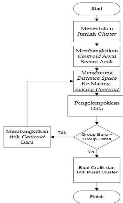
Gambar 2.2 Diagram Alur Implementasi Algoritma K-Means
