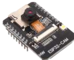
**Gambar 2.1 Esp32-cam**
