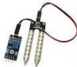
**Gambar 2.1** Soil Moisture Sensor
