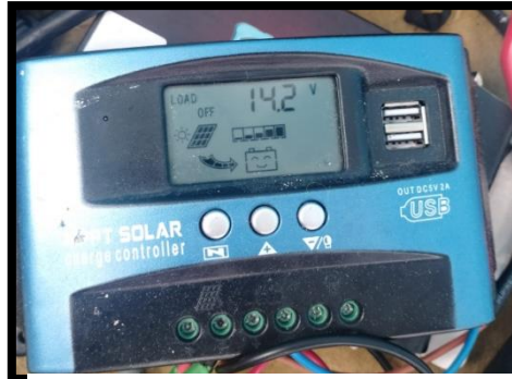
Gambar 3. 9 SCC (Solar Charger Controller)
