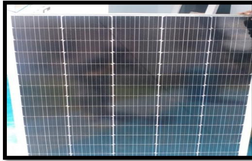
Gambar 3.1 panel surya monocrystalline
