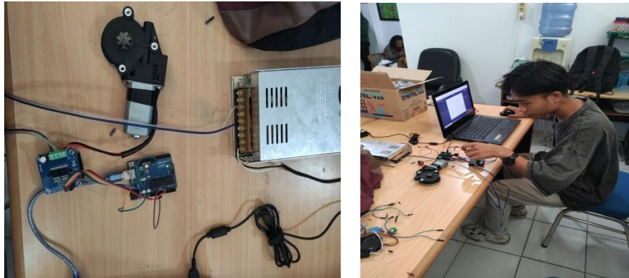
Gambar 4. 1 Perancangan motor power window dan driver motor BTS7960 .
