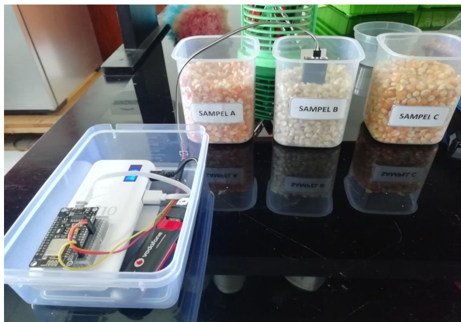
Gambar 4.7 Proses pengukuran kadar air langsung
