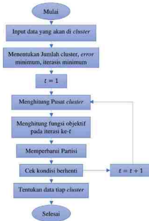
Gambar 2. 2 Flowchart algoritma Fuzzy C-means
